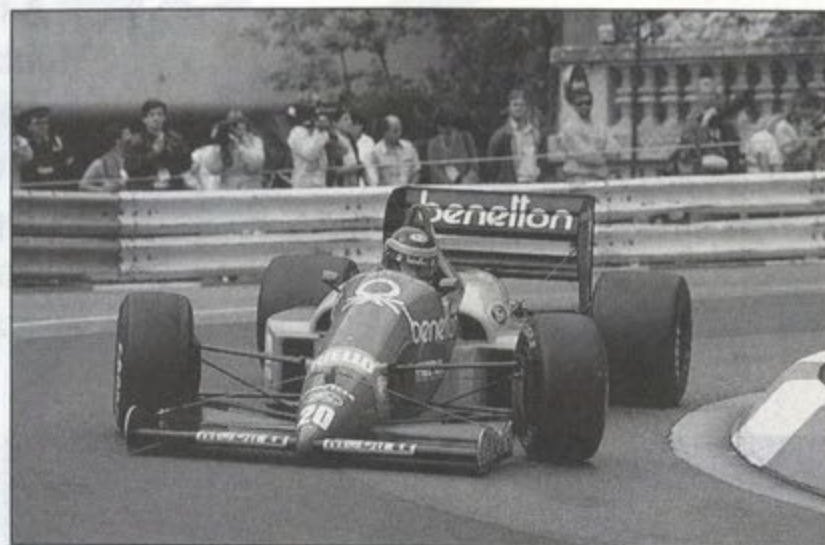
A Benetton B188 taking a tight hairpin at Monaco. The lock is often increased on cars on this circuit to cope with this first gear left-hander.
