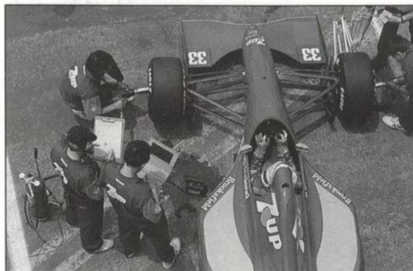
Race mechanics set-up a Jordan 191 at the Mexican Grand Prix. The driver must sit in the cockpit fully kitted up and the fuel tanks must be half-full.
