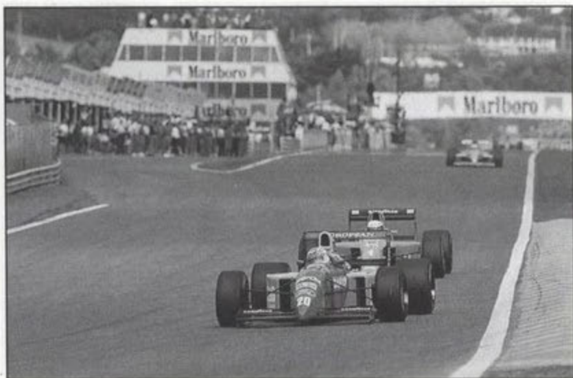
The rear car 'slipstreams' the car in front of it on the straight in the Portuguese Grand Prix; 'getting a tow' prior to overtaking.
